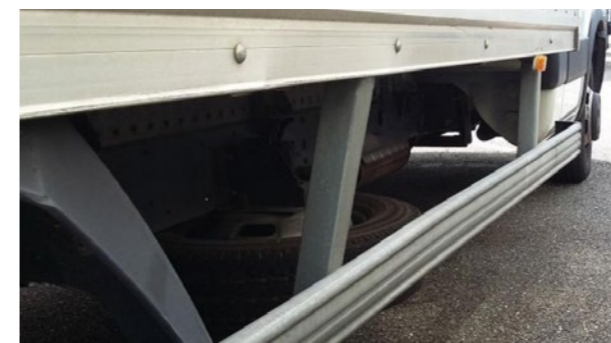
Side underun guards: Deformation within economic repair
