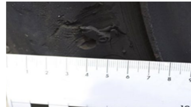
Tyres: Notch > 3 mm deep, removal
