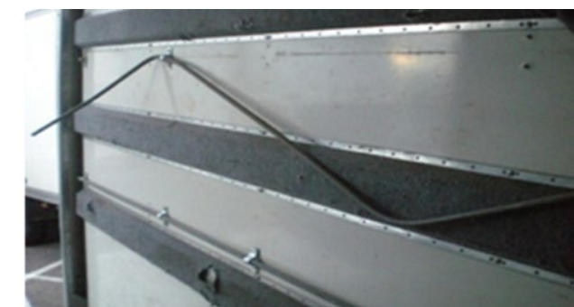
↻ Upholstery and rods: Rods, fastenings, upholstery missing or deformed beyond economic repair
