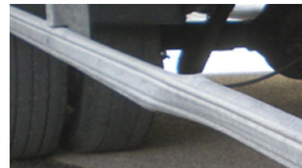
Side underun guards: Deformation beyond economic repair
