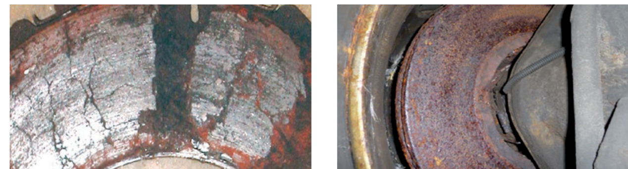
Rusted, ground, worn brake discs
